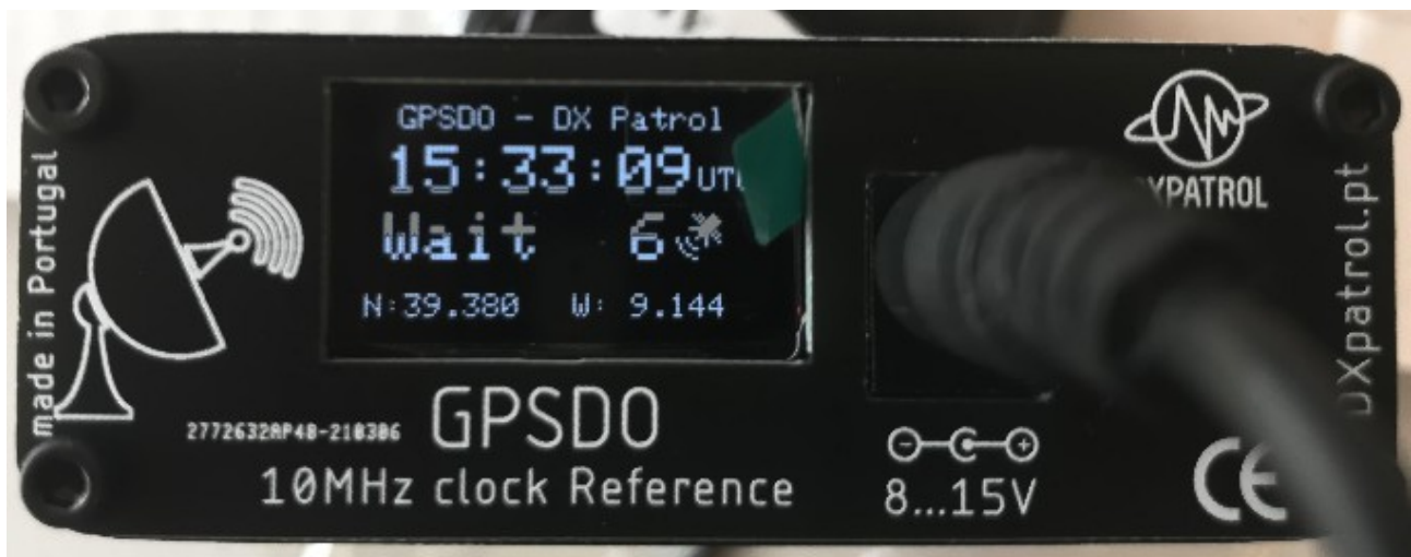
Fig 7: 6 satellites in range, clock and coordinates detected. OCXO warming up.
