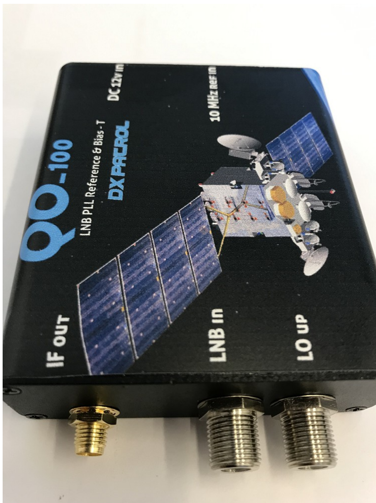
Fig9 F-connectors and SMA
